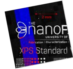
~ 2.7 x 1.4 mm Ti 2p (red) and 5.5 x 1.4 mm Si 2p (blue) chemical map overlaid with SXI image
