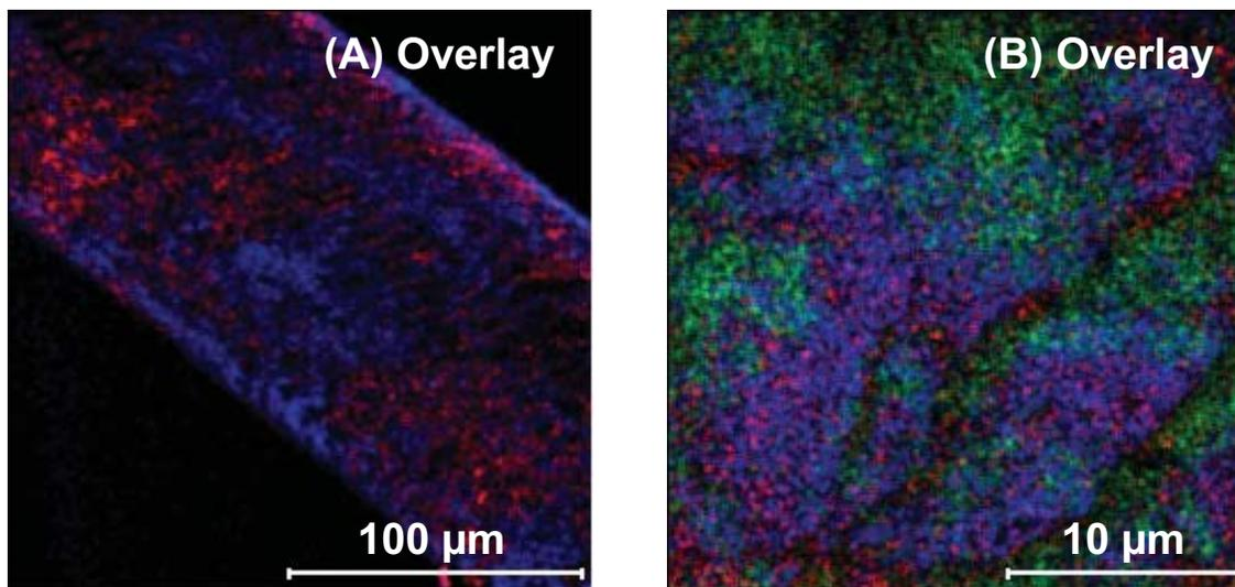
Figure 4: Color overlay images reveal the relative distribution of chemical components on the surface of the hair. (A) 200 μm FOV overlay of  $\text{C}_{16}\text{H}_{33}\text{O}_2^+$  (257 m/z, red) and  $\text{Ca}^+$  (40 m/z, blue). (B) 25 μm FOV overlay of  $\text{Na}^+$  (23 m/z, red),  $\text{Ca}^+$  (40 m/z, green) and  $\text{CN}^-$  (26 m/z, blue).
