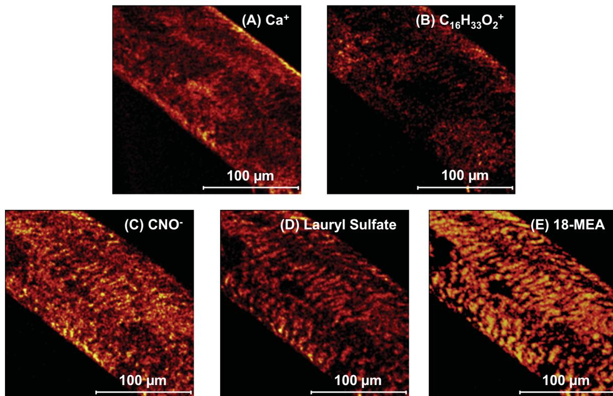
Figure 3: A complete chemical picture of the hair surface is provided by a set of molecule-specific and elemental images. (A) Calcium ( $\text{Ca}^+$ , 40  $m/z$ ). (B) Acid hydrate ( $\text{C}_{16}\text{H}_{33}\text{O}_2^+$ , 257  $m/z$ ). (C) Amino acid ( $\text{CNO}^-$ , 42  $m/z$ ). (D) Lauryl sulfate ( $[\text{M-O}+\text{C}_2\text{H}_4]$ , 293  $m/z$ ). (E) 18-MEA ( $\text{M}$ , 341  $m/z$ ). The field-of-view in each image is 200  $\mu\text{m}$  x 200  $\mu\text{m}$ .
