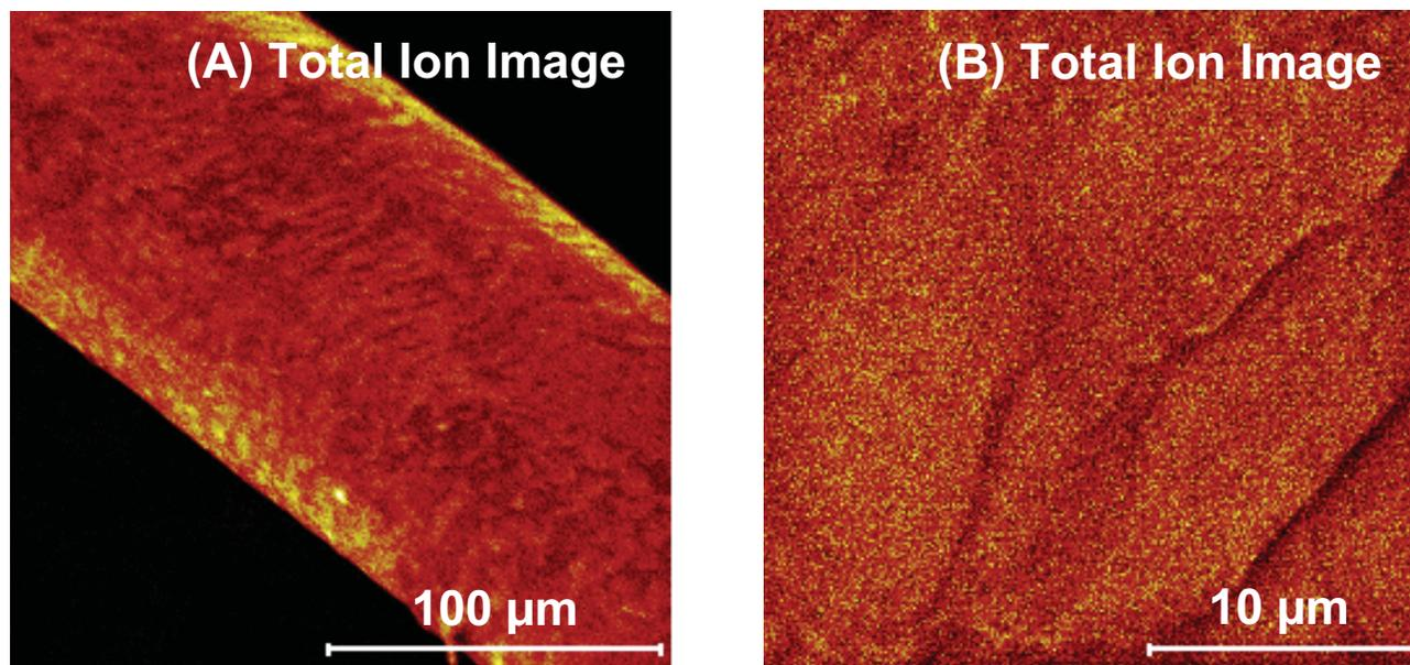
Figure 1: Images of a human hair show the ability of the PHI *nanoTOF* to collect information from the entire curved surface that is visible to the analytical ion beam. Individual cuticles are observable along the hair shaft, and the high magnification image demonstrates the spatial resolution provided by the *nanoTOF*. (A) Total ion image (-SIMS, 200 µm FOV). (B) Total ion image (-SIMS, 25 µm FOV).
