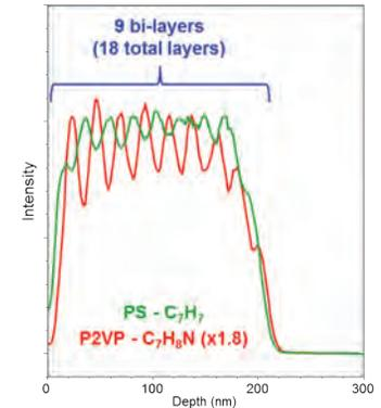
A depth profile of a poly(styrene)/poly(2-vinyl pyridine) (PS/P2VP) copolymer blend approximately 200 nm-thick on a Si substrate. The profiles and 3D image data expose the 3-dimensional structure and composition.
