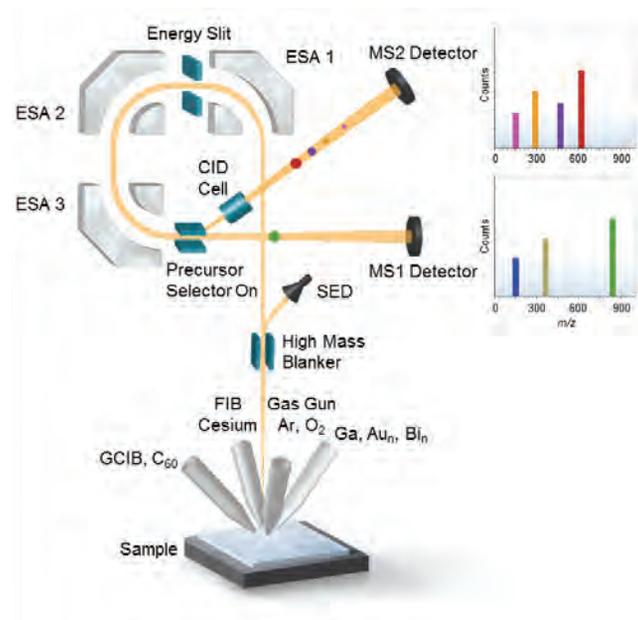
The schematic highlights the triple electrostatic analyzer (ESA) design of the *nanoTOF II*'s TRIFT mass spectrometer. Selected precursor ions are deflected at high energy into a collision-induced dissociation (CID) cell for fragmentation. The product ions are collected at the  $MS^2$  detector. Any ions not within the monoisotopic precursor selection window continue on their original flight path to the  $MS^1$  detector.
