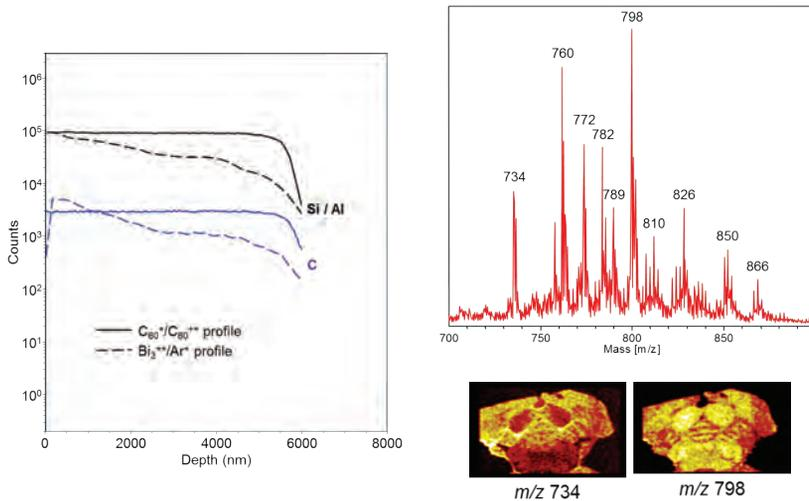
(LEFT) Depth profiles of a 6  $\mu\text{m}$ -thick aluminosilicate sol-gel on copper by Ar and C<sub>60</sub> sputtering. The C<sub>60</sub> ion beam does not produce the differential sputtering artifacts produced by the Ar ion beam. Additionally, the C<sub>60</sub> analysis beam does not produce the surface transient artifact that is produced by the Bi analysis beam.
