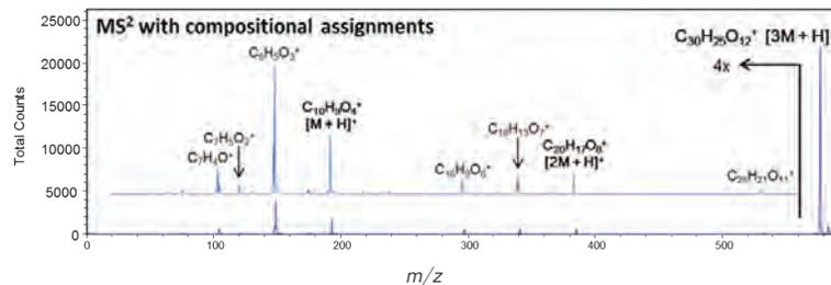
The utility and effectiveness of Parallel Imaging MS/MS is demonstrated in the analysis of surface precipitates on heat-treated poly(ethylene terephthalate) (PET). In only a 13 minute acquisition the 3 to 7  $\mu\text{m}$  precipitates are observed and the tandem mass spectrum clearly identifies the molecular composition of the precipitates. The lateral resolution in both the  $\text{MS}^1$  and the  $\text{MS}^2$  images is measured to be < 200 nm.
