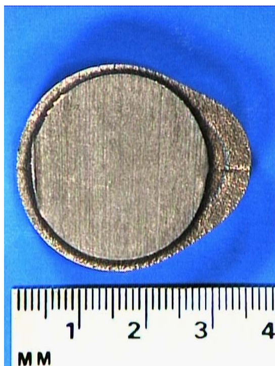
Figure 1. Side view of cam lobe. Note the circular cross section of the cam shaft.
