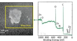
A micro area spectrum from the smaller features, obtained using a 10  $\mu m$  diameter x-ray beam, identifies
