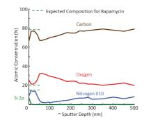
10 keV  $C_{60}$  depth profile of a 50/50 rapamycin and PLGA film showing segregation of the rapamycin to the surface of the coating.
