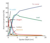
2 keV Ar sputter depth profile of the surface species on a solder ball used for semiconductor packaging
