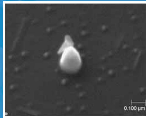
Secondary electron image of a silicon nanocone.
