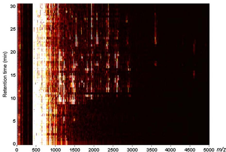
**Fig. 4 – Reconstructed LC trace displaying full mass spectra in a time resolved manner. Peaks corresponding to digested peptides especially above 1000  $m/z$  and up to 5000  $m/z$  show up only when they are eluted from the LC column.**
