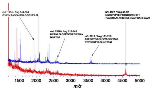
**Fig. 3 – Mass spectra of fractions #29 (bottom) and #44 (top). Peptide sequences are detected up to 5 kDa.**
