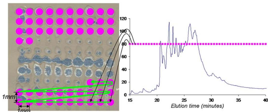
**Fig. 1 – Scheme of the nanoLC fraction deposition on the 2,5-DHB-coated plate. 15 min after injection fractions start to be deposited in a 10-by-10 array using a fly-back pattern. After 20 min, peptides start to be eluted from the column, as can be seen from the UV trace on the right.**
