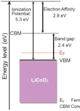
The full energy diagram can be obtained using **UPS/LEIPS**. LEIPS uses a low-energy electron beam, which ensures damage-free energy diagram evaluation! Performing XPS and UPS/LEIPS in the same area provides a direct link between chemical properties and electronic structure of the electrolyte/electrode interface.
