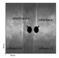
Secondary X-ray induced Electron (SXI) imaging using 10  $\mu$ m X-ray spot in XPS is used to locate lithium/electrolyte interface.
