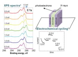
Operando XPS can probe the evolution of the chemical structure and the surface potential at the electrode/electrolythe interface of lithium-ion batteries under electrochemical conditions.
