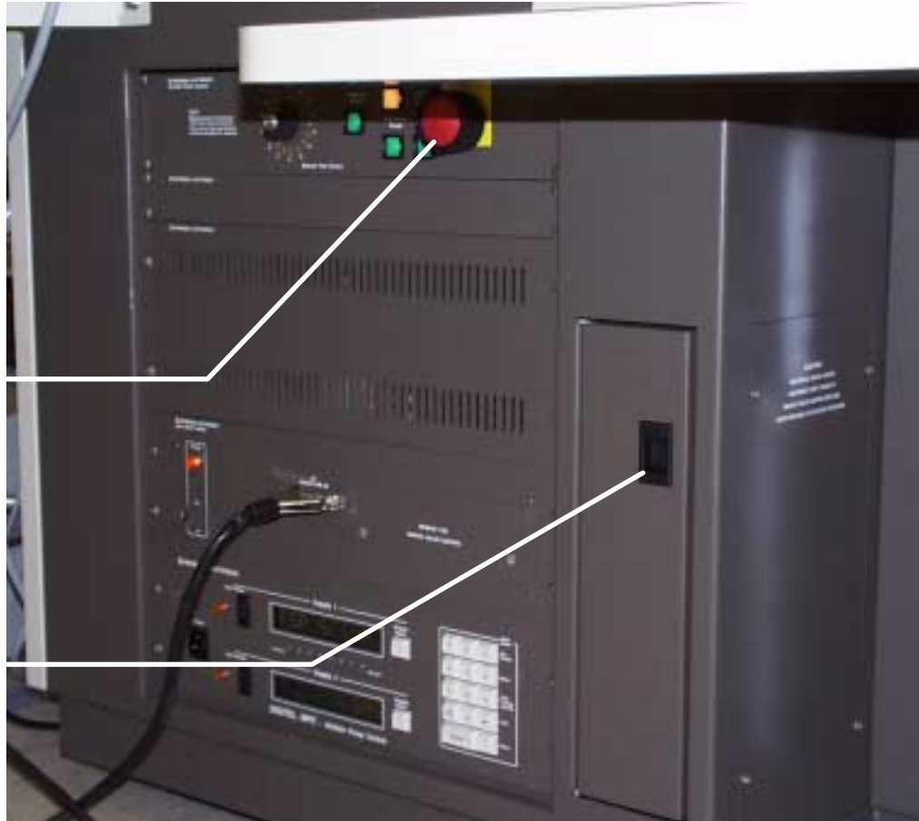
Front view of 5801 system console showing the location of the circuit breaker panel and the emergency off button.
