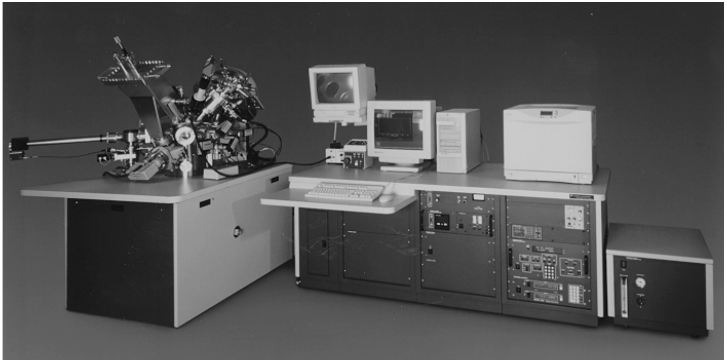
Photograph of the 5802 dual console MultiTechnique XPS system.
