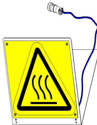
Figure 10-1. Installation of the Bakeout Warning Sign is required prior to starting the bake.
