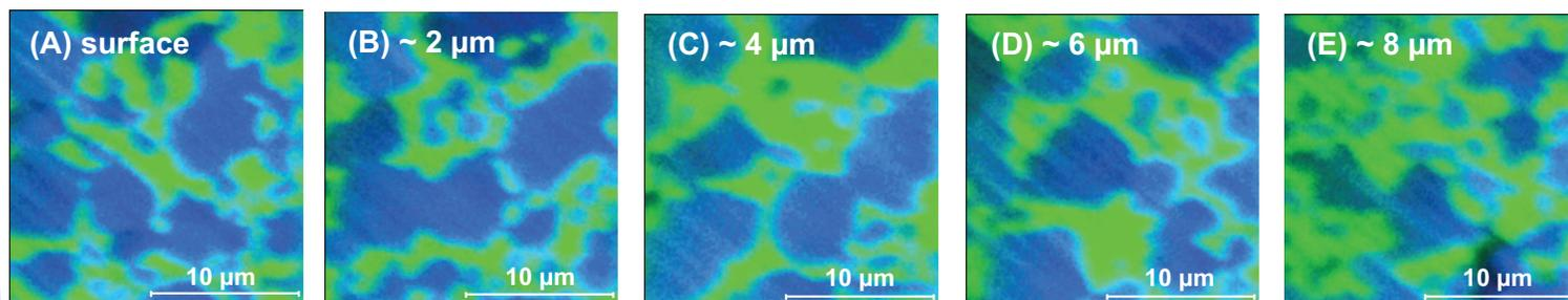
Figure 2: A set of 2D images-at-depth showing the Cu and W phases of the sample as color overlays of the  $\text{Cu}^+$  (green, 63  $m/z$ ) and  $\text{WO}^+$  (blue, 200  $m/z$ ) images. The field-of-view (FOV) in each image is 20  $\mu\text{m}$  x 20  $\mu\text{m}$ .
