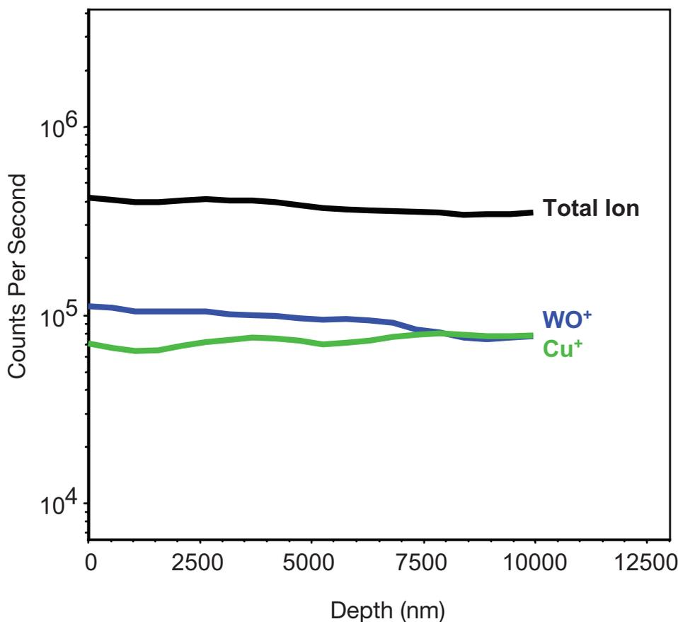
Figure 3: Concatenated depth profile, generated from the 20 individual RAW data stream files, showing the profiles of  $\text{Cu}^+$  (green, 63 m/z),  $\text{WO}^+$  (blue, 200 m/z), and the total ion signal. Note that the depth scale is defined by the cumulative length of the FIB line cuts in the plane perpendicular to the surface of the sample (see Figure 1B).
