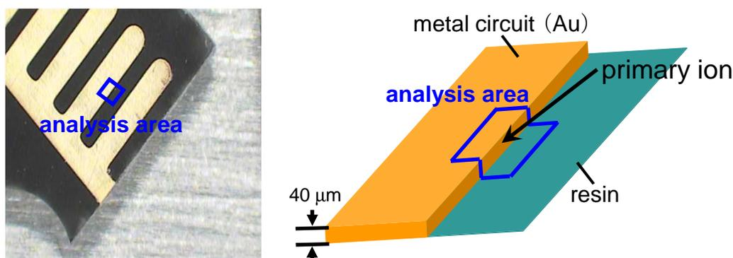
Figure 1. (LEFT) Optical microscope image of a metal interconnect structure on a flexible substrate that was obtained from a consumer product. An approximately  $200\ \mu\text{m} \times 200\ \mu\text{m}$  field-of-view is shown. (RIGHT) A schematic illustration of a gold interconnect on a flexible substrate where the approximated analysis area has been indicated.
