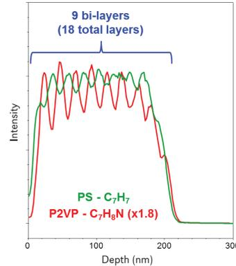
A depth profile of a poly(styrene)/poly(2-vinyl pyridine) (PS/P2VP) copolymer blend approximately 200 nm-thick on a Si substrate. The profiles and 3D image data expose the 3-dimensional structure and composition.
