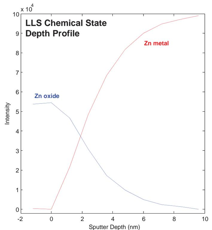
Figure 2: Chemical state Auger depth profile showing the presence of a thin Zn oxide layer on a Zn metal surface.
