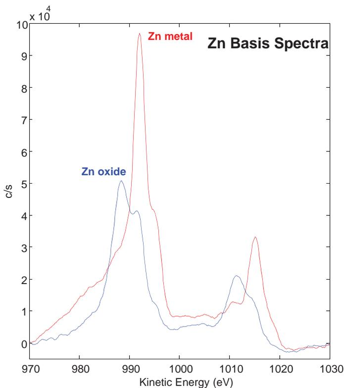
Figure 1: High energy resolution (0.1%) Zn basis spectra for Zn metal and Zn oxide extracted from the depth profile data set as part of the Linear Least Squares (LLS) fitting process used to create the chemical state depth profile shown in Figure 2.
