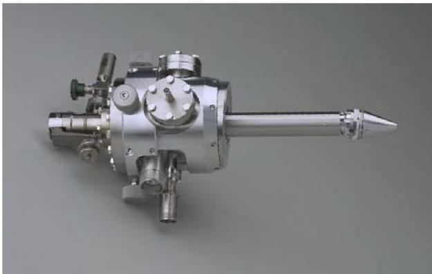
This approach to charge neutralization is possible with Physical Electronics Auger systems equipped with the 06-350 floating column ion gun. This ion gun forms ion beams down to a few eV, with useful ion currents. The ion gun will also operate at voltages up to 5 kV for sputter depth profiles at high sputter rates. The ion column has a 5° bend to eliminate neutrals. The gun is fully digitally controlled and offers stored user settings for the ultimate in experimental reproducibility.
