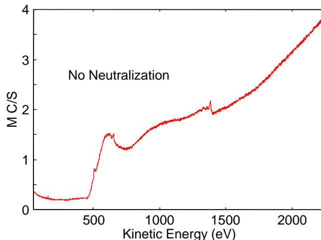
In this example, an Auger spectrum was acquired from an area near the center of an Al bond pad is surrounded by polyimide. The spectrum was adversely modified by the charge on the surrounding polyimide, resulting in a lack of useful information in the Auger spectrum below approximately 1000 eV. Note that the higher energy Al Auger peak occurs at the correct energy, but appears attenuated in intensity.
