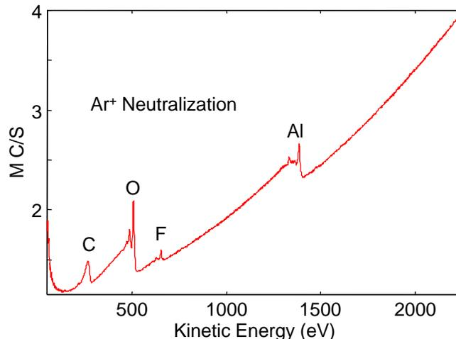
A low energy argon ion beam may be effective in reducing or eliminating surface charge. In the example shown above, a 70 eV Ar<sup>+</sup> ion beam was used during Auger analysis to eliminate the charge on the polyimide surrounding the bond pad. This made it possible to obtain a normal Auger spectrum from the bond pad. The effectiveness of argon ion neutralization may be affected by changing the ion energy, ion current, and the flood area.
